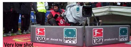
of this system is that contrary to other cameraseat systems, the seat is not directly connected to the center column. Almost no shock motion is transmitted from the operator to the camera as the camera column is not loaded by the operator's weight. The unlinked rotation on the same axis also avoids unwanted movement of the camera when moving the seat.
