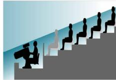
The Orbiter allows independent movement of camera and seat, on the same axis. There are two remarkable and patented features of this system. Contrary to other cameraseat systems, the seat of the Orbiter is not directly connected to the camera column. Hence no shock motions are transmitted from the operator to the camera. The unlinked rotation on the same axis also avoids unwanted movement of the camera when moving the seat.
